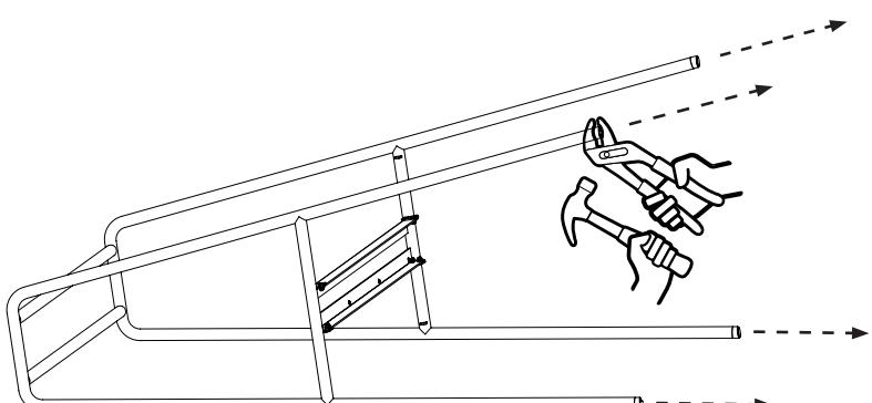
3. Hold the nuts with the wrench and remove the screws from the stretcher.
